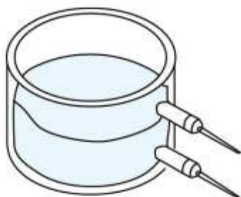
图1、液位测量—塑料或玻璃器皿 liquid level measurement--plastic or glass container
